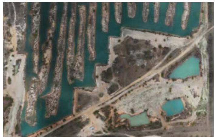
Drone aerial view of Marlboro Sand and Gravel's Airport Mine showing finger islands created from previous dragline mining.
